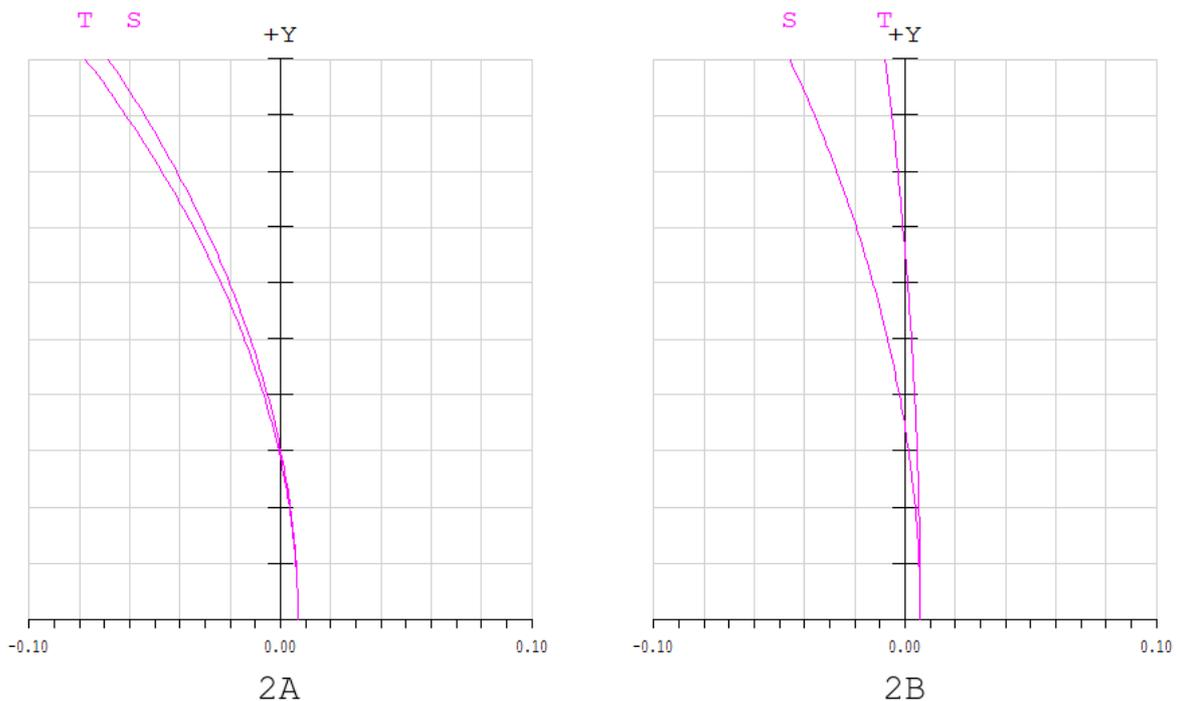
Figure 2: Field curvatures before (2A, left) and after (2B, right) defocusing. Defocusing bends tangential field curvature towards flat.
