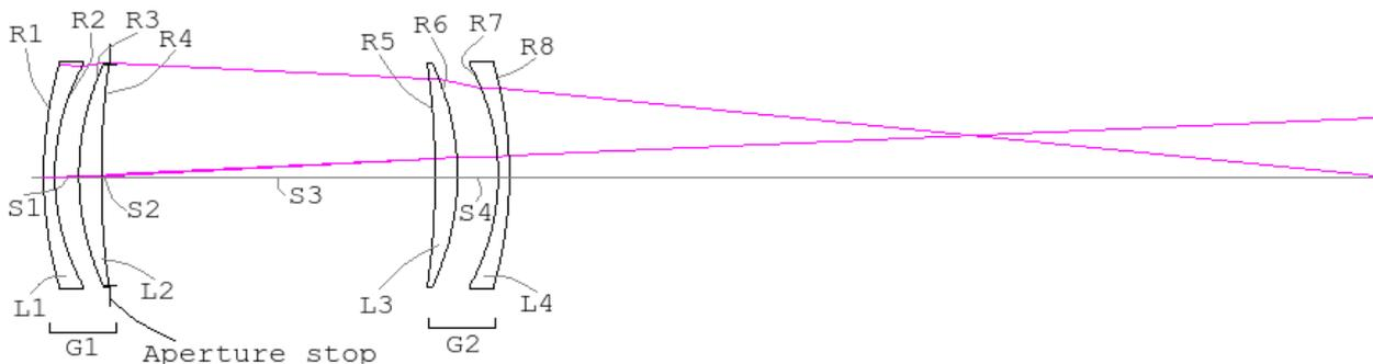
Figure 1: Layout of a  $f=100$  mm system with chief and marginal rays.
