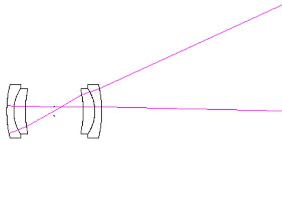
Figure 3: A basic rapid rectilinear camera lens layout.
