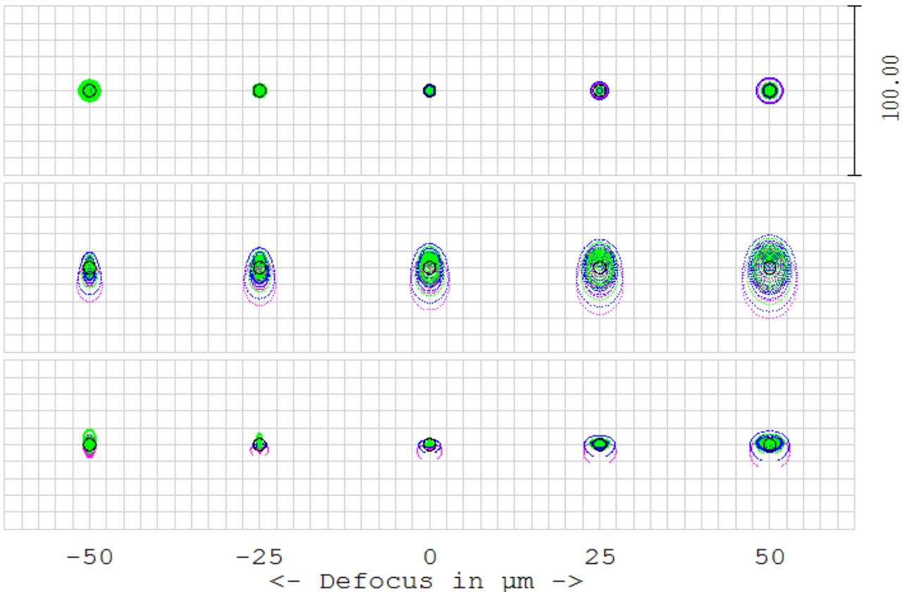
Figure 4: Spot diagrams through focus for axial image (top), and edge image (FFOV  $6^\circ$ ) where lens group focal lengths are equal (middle), and where lens group focal lengths differ by a factor of 0.944 (bottom). The term defocus in the graph refers to image plane defocus, not the lens group defocus used in this paper.
